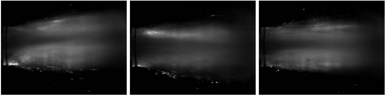
Figure 4: Three frames of video \sim 1.33 ms apart show a typical oscillating spray.
