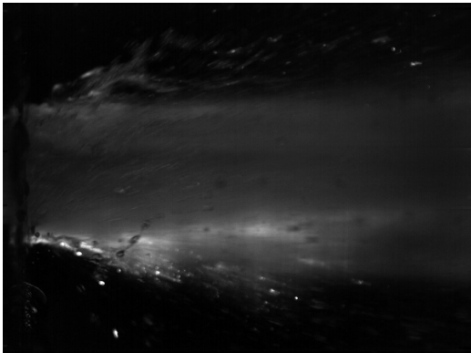
Figure 5: An image a spray with axisymmetric pulsing—an increased cone angle is caused by ligaments outside the main spray core.
